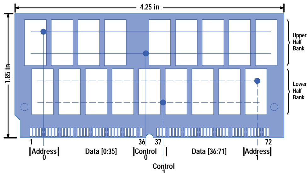
The motivation for designing our own memory module rather than using an industry-standard SIMM was memory capacity and performance. We would have needed twice as many PC SIMMs for an equivalent amount of memory. This would create a physical space problem because twice as many connectors would be needed, and would create performance problems because of the increased printed circuit board trace lengths and unterminated transmission line stubs.
