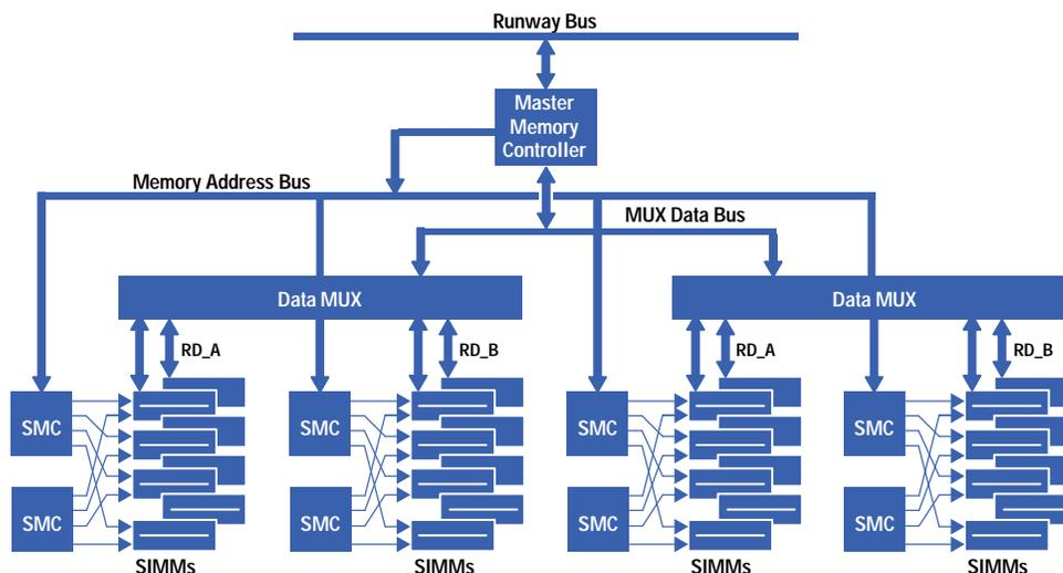
In an entry-level workstation, the memory can start at 32M bytes (one pair of SIMMs with 4M-bit DRAMs) and be expanded up to 512M bytes (using 4 pairs of SIMMs with 16M-bit DRAMs) as shown in Fig. 1. The HP 9000 J-class workstation can be expanded to 1G bytes of memory using eight pairs of SIMMs with 16M-bit DRAMs. The HP 9000 Model K400 server can be expanded up to 2G bytes using 16 pairs of SIMMs with 16M-bit DRAMs installed in two memory carriers.
