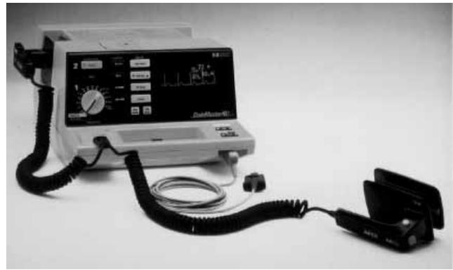
**Fig. 2.** An HP CodeMaster defibrillator with SpO<sub>2</sub> channel.
