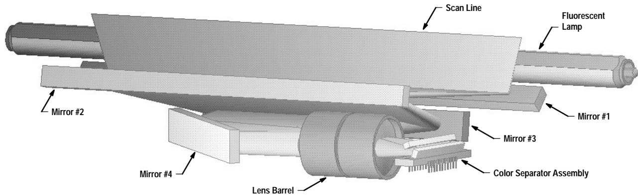
**Fig. 6.** Mechanical design layout of the HP ScanJet 3c/4c optical path. The light path is from the scan line to mirror #1 to mirror #2 to mirror #3 to mirror #4 to the lens to the color separator to the CCD detector.
