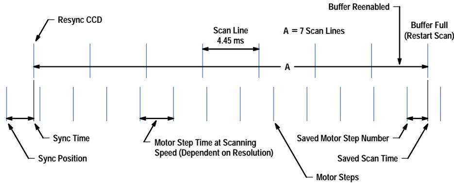
**Fig. 10. Start-stop timing.**
