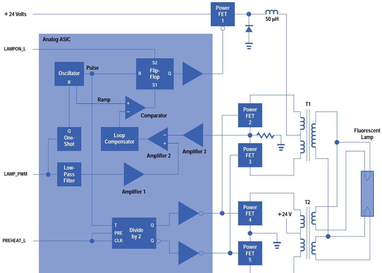
**Fig. 8.** Block diagram of the fluorescent lamp driver.
