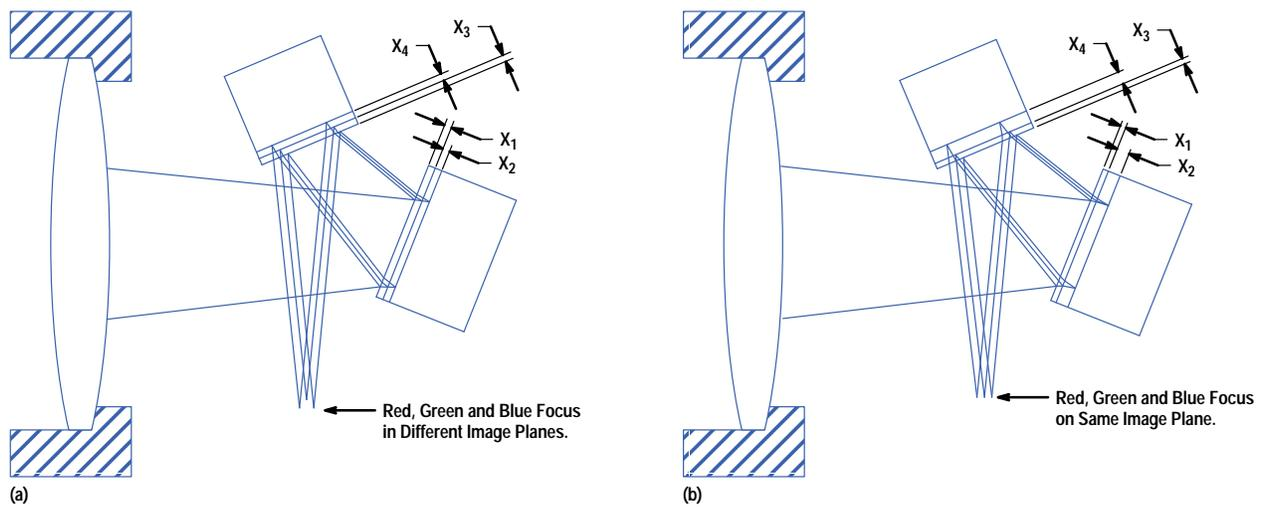
**Fig. 4.** (a) Chromatic aberration of an uncorrected system.  $X_1 = X_2 = X_3 = X_4$ . (b) To ensure that simultaneous focus for red, green, and blue is achieved in the HP ScanJet 3c/4c scanner, unequal path lengths are used to compensate for the chromatic aberration of the lens.  $X_1 = X_3$  and  $X_2 = X_4$ , but  $X_2 \neq X_1$ .
