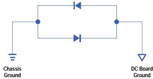
**Fig. 12.** Diode connection for ESD and RFI suppression.
