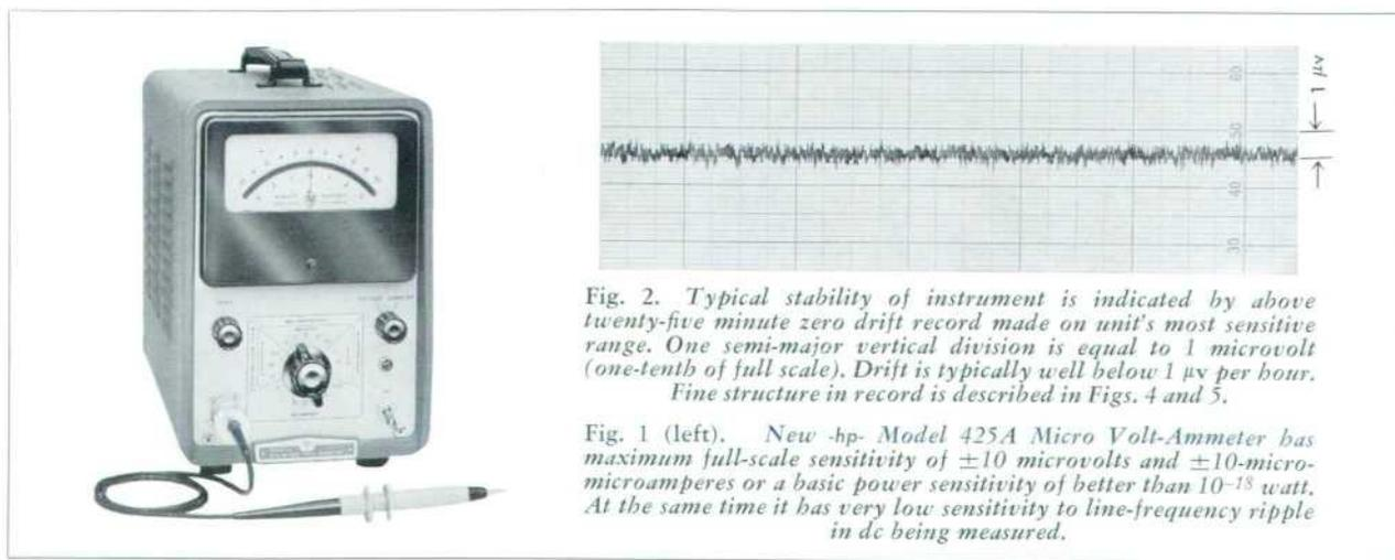
Fig. 2. Typical stability of instrument is indicated by above twenty-five minute zero drift record made on unit's most sensitive range. One semi-major vertical division is equal to 1 microvolt (one-tenth of full scale). Drift is typically well below 1  $\mu$ v per hour. Fine structure in record is described in Figs. 4 and 5.
