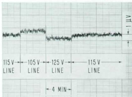
noise readings are almost undetectable. The record is arranged so that one semi-major chart division corresponds to one major division on the meter face, i.e., 1 microvolt in Fig. 4 and 3 microvolts in Fig. 5.
