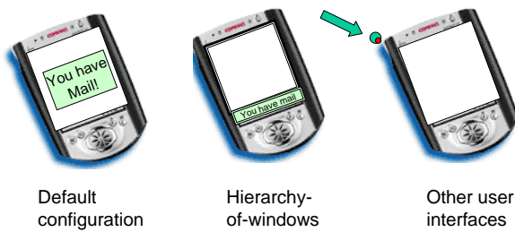
Figure 12: Other energy-adaptive designs. The picture on the left illustrates a base system. The system in the middle uses two display panels to provide coarse-grain adaptivity for power. The right picture shows how display power for low-content messages can be reduced by using simpler visual or non-visual cues.
