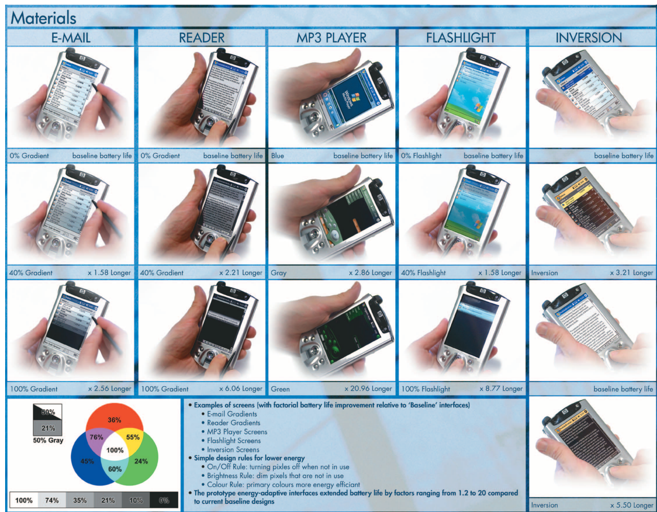
Figure 3. Energy-aware user interfaces. The images labeled "baseline battery life" represent the default interface, while the other images show the energy-aware interfaces. The energy values for various configurations and the rules used to guide the design of the energy-aware interfaces are summarized at the bottom of the picture.
