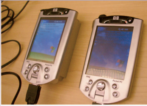
Figure 2. Energy-adaptive display design. The device on the left is a prototype iPAQ with an OLED display. For comparison, a similar device with a conventional LCD is shown on the right. OLED displays provide one way of enabling the fine-grained control of display power needed for an energy-optimized design.
