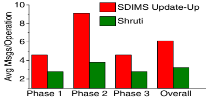
Fig. 13. Temporal heterogeneity: Average message count per operation in Shruti vs. SDIMS for three phases of the experiment.
