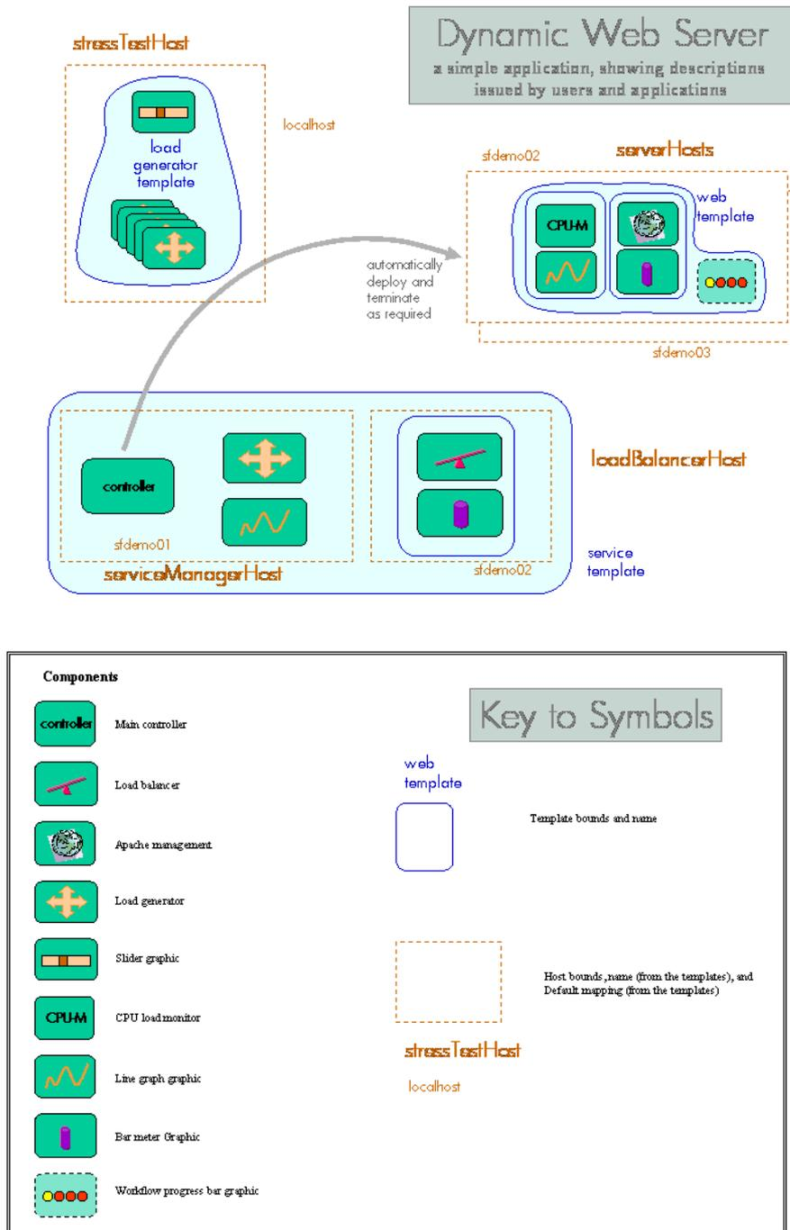
The diagram above is an outline of the various parts of the demonstrator. The three main parts, described as different SmartFrog templates, are the core service (the service manager and the load balancer), the web server(s), and the load generators that are provided so as to provide sufficient simulated load to cause the service to have to adapt.
