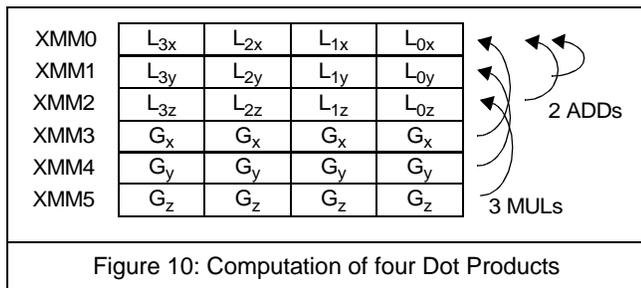
Figure 10: Computation of four Dot Products
