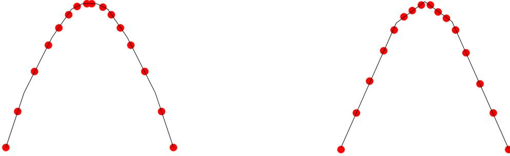
Figure 2: Polygonal up-sampling of arbitrarily pre-sampled curves.
