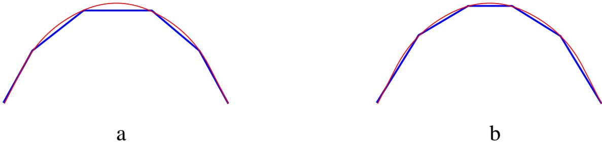
Figure 1: Invariant grids on a curve: a. Euclidean arclength, b. affine arclength
