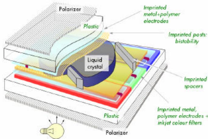
Figure 2: Layout of the HP prototype of a bistable plastic display
