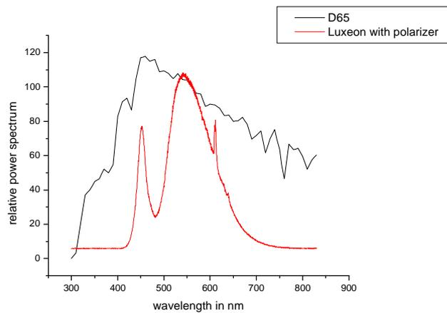
Figure 3: D65 spectrum and spectrum of a Luxeon backlight in combination with a polarizer.
