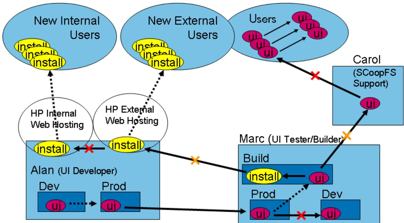
Figure 2. The SCoopFS development and deployment network with those elements not supported by Microsoft Live Mesh removed. The two orange x's represent either a violation of POLA or a usability failure that causes the user to have to work around inadequacies in the software. The three red x's represent failures of functionality, or a violation of POLA so severe it results in a full breach of all the machines in a subnetwork.
