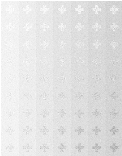
Figure 2. Scaled representation of the void pantograph test sheet. Actual size is 7" W by 9" H at 600 ppi.
