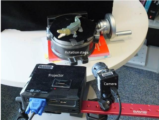
**Figure 2:** set up of scanner and stage
