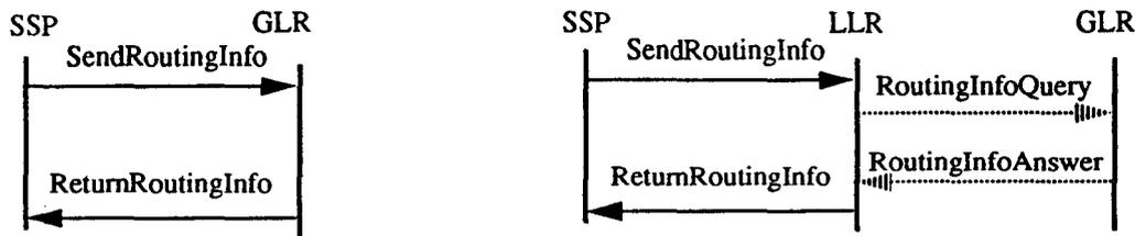
Figure 3- Signalling flow for Call-Setup in architectures 1, 2 (left) and 3 (right)
