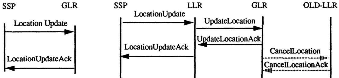
Figure 4- Signalling flow for Registration in architectures 1, 2 (left) and 3 (right)
