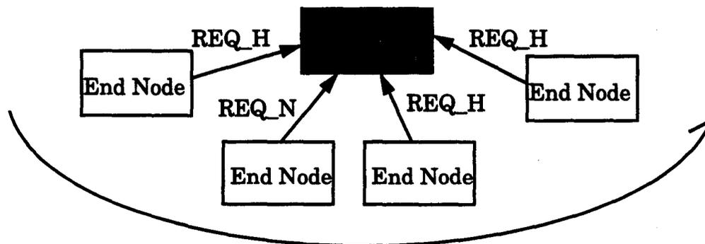
**Figure 8 The Hub uses a Cyclic order of servicing Requests from End Nodes. High priority Requests take precedence over Requests at Normal priority.**
