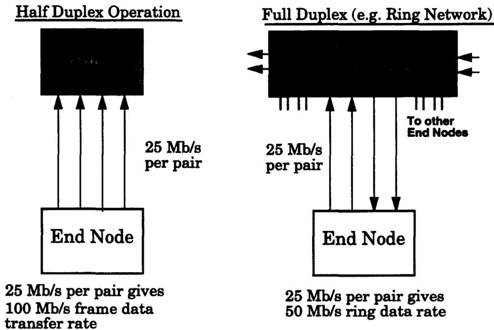
**Figure 1 The advantage of Half Duplex Link Operation as opposed to Full Duplex Link Operation. Assumes 25 Mb/s transmission on each Category 3 cable physical layer.**
