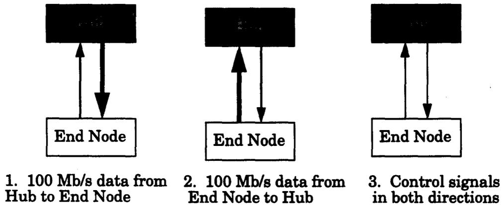
**Figure 3 The Link Protocol States in Dual Simplex Operation**
