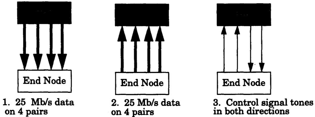
**Figure 2 The Link Protocol States in Half Duplex Operation**
