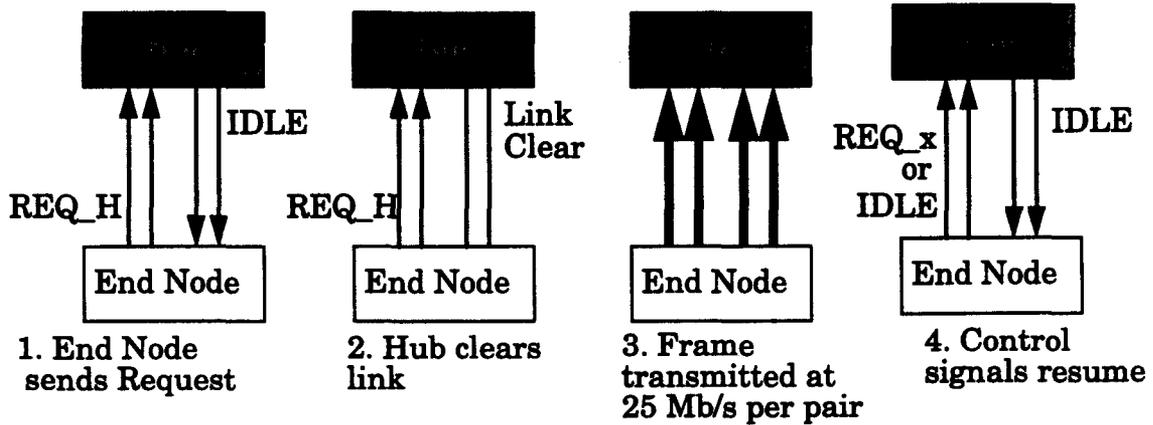
**Figure 4 Link Protocol Sequence of the End Node transmitting a Frame**
