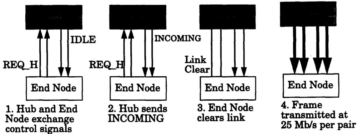
Figure 5 Link Protocol Sequence of the End Node receiving a Frame
