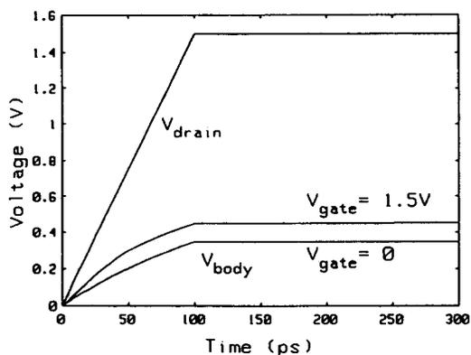
Fig. 1 Transient Simulation: The drain voltage is ramped from zero to 1.5V in 100 ps and then held constant.  $V_{body}$  follows due to capacitive coupling to the drain. In this example impact ionization has no effect.
