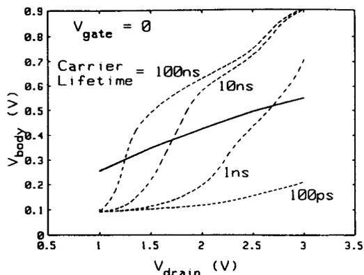
Fig. 2 Comparison of transient and DC: Transient = solid line; DC = dashed line. For the transient case, the  $V_{drain}$  ramp time is 100 ps in all cases and the  $V_{body}$  is measured at  $t = 300$  ps.  $V_{body}$  (transient) does not depend on impact ionization or carrier lifetime.
