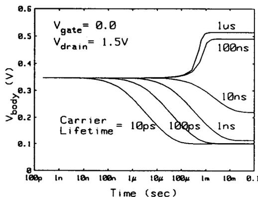
Fig. 4 Time Evolution of  $V_{body}$ . This figure continues the time axis of the simulation in Fig. 1.
