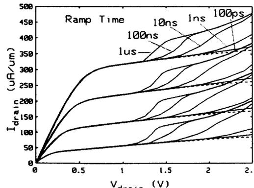
Fig. 6 Transient IV Characteristics.  $V_{drain}$  is ramped from zero to 2.5V in varying times for  $V_{gate} = 0.75, 1.0, 1.25$  and 1.5 V. Dashed lines are for no impact ionization.
