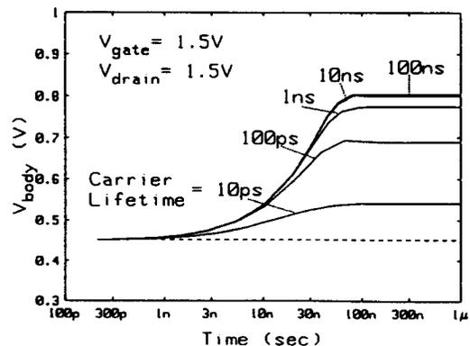
Fig. 5 Time Evolution of  $V_{body}$ . This figure continues the time axis of the simulation in Fig. 1. Dashed line is for no impact ionization.
