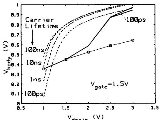
Fig. 3 Comparison of transient and DC. Transient = solid line; Transient without impact ionization = symbols; DC = dashed lines. For the transient cases, the  $V_{drain}$  ramp time is 100 ps in all cases and the  $V_{body}$  is measured at  $t = 300$  ps.
