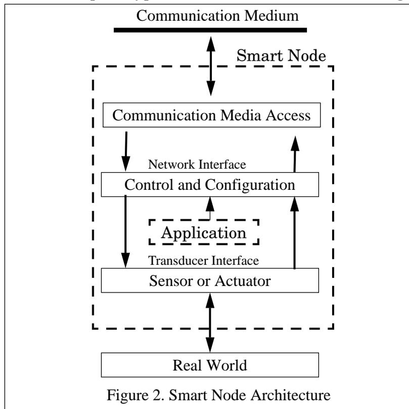
The Communication Media Access block handles the low-level protocol required to access the physical medium. Included in this block, is a media-dependent transceiver. This transceiver is the physical interface to the medium. Ideally, the interface between this block and the Control and Configuration block, i.e., the network interface, is media and protocol independent.
