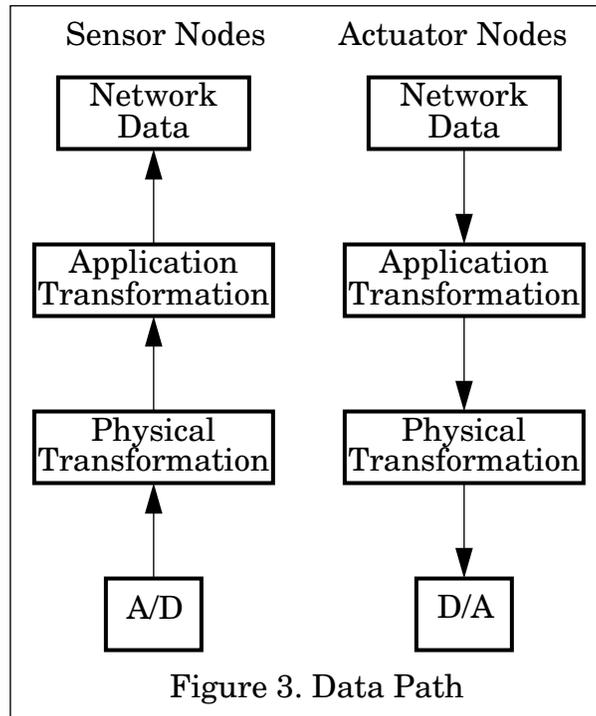
The physical transformation converts between the digital representation in the International System of Units, SI, and the raw digitized representation provided by the transducer. This conversion is based on information from the “electronic data
