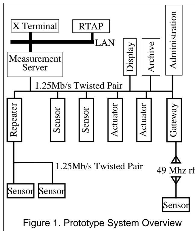
A variety of communication media are used in the demonstration system. An Ethernet LAN is used in the traditional portion of the system. A 1.25Mb/s twisted pair and a 49Mhz low-power RF link are used for communication in the distributed portion of the system. A repeater is shown to illustrate the segmentation of the network allowing more nodes than permitted with a single twisted pair.
