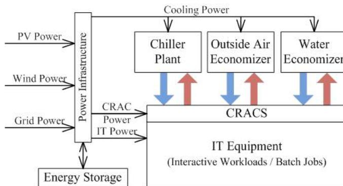
**Figure 2: Micro-grid Based Infrastructure**
