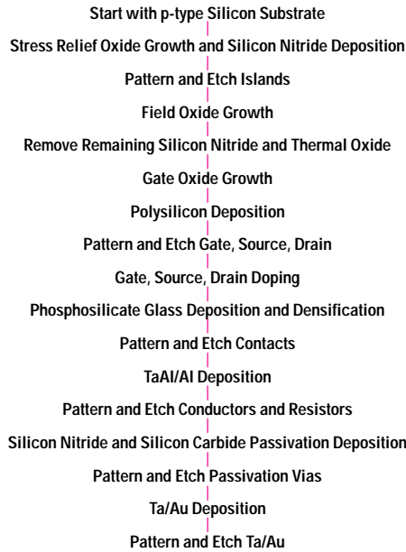
Fig. 5. Integrated driver printhead process flow.
