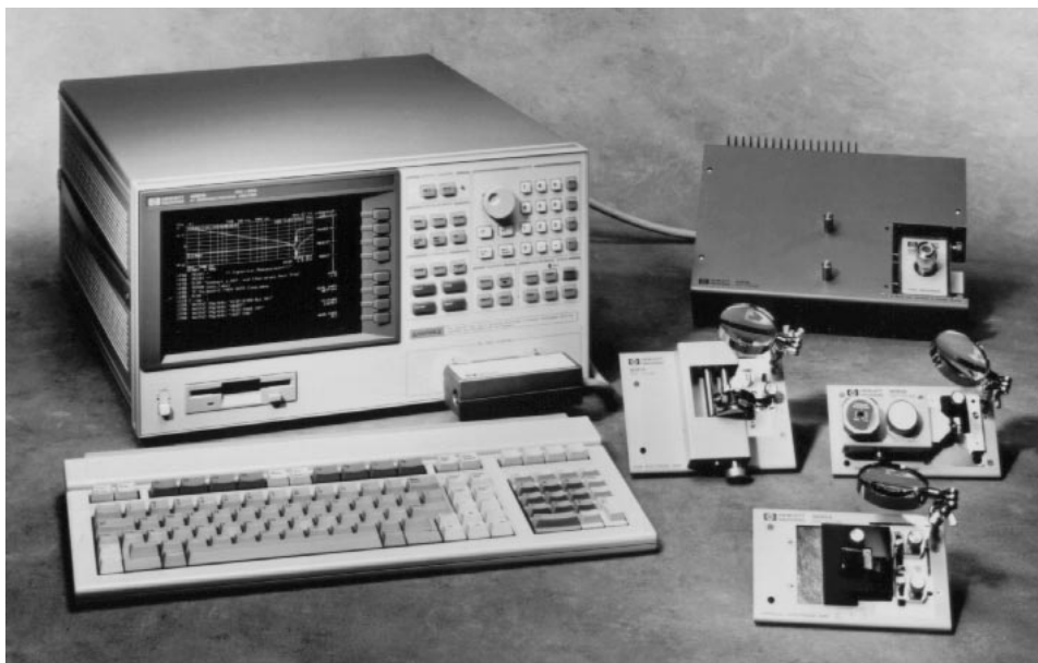
Fig. 1. The HP 4291A RF impedance analyzer measures impedances of components and materials at frequencies from 1 MHz to 1.8 GHz. New surface mount test fixtures and built-in calibration and compensation routines ensure accuracy.
