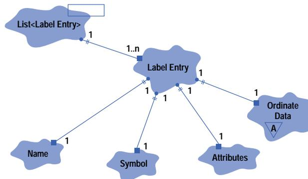
**Fig. 4.** Class diagram of the label entry class using Booch notation.<sup>1</sup>
