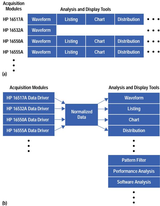
**Fig. 1.** (a) In the HP 16500A/B logic analysis system coding model, tool software had to be rewritten for each plug-in card. (b) In the HP 16505A prototype analyzer coding model, data is normalized immediately after acquisition and is available to all tools in a standard format. Thus, the tools had to be coded only once.
