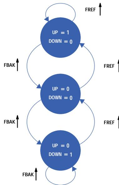
**Fig. 3.** State table for the phase-frequency detector.
