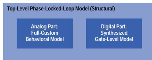
**Fig. 2.** Structure of the phase-locked loop model.
