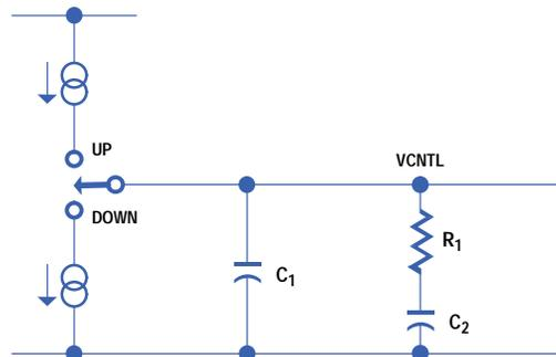
**Fig. 4.** Simplified charge pump and filter model.
