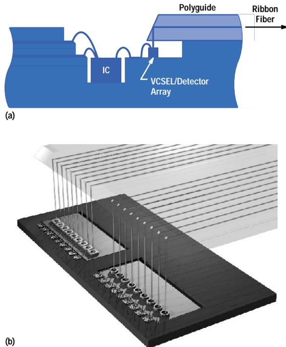
interface allows the VCSELs and detectors to be packaged in close proximity to the transceiver ICs, allowing control of electrical parasitics and GHz-bandwidth operation. Because the waveguides are multimode, simultaneous alignment of ten channels to the VCSEL and detector arrays is possible with loose alignment tolerances.
