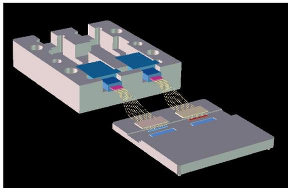
The design of the optical-electrical interface is shown in **Figure 4**. The VCSEL and detector arrays are packaged with the transceiver ICs in a 324-pin ceramic BGA package. Polyguide waveguides couple light between the VCSEL and detector arrays and the ribbon fiber using 45° out-of-plane mirrors and fiber-to-waveguide connectors. The ceramic package features impedance-controlled traces and integrated resistors for termination of input ECL signals. The use of a 45° optical
