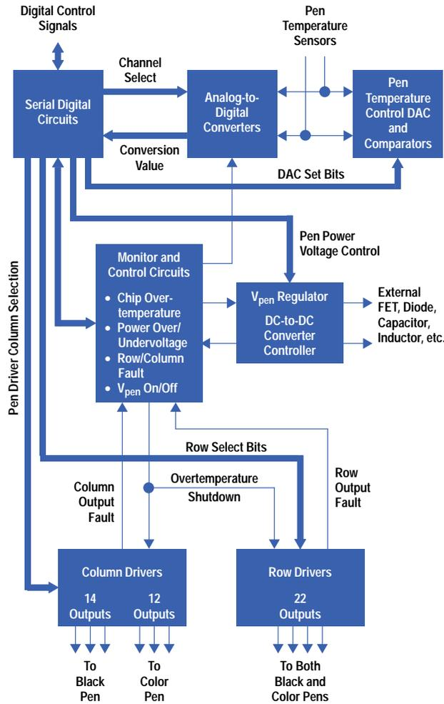
**Fig. 2.** Block diagram of the mixed-signal ASIC.
