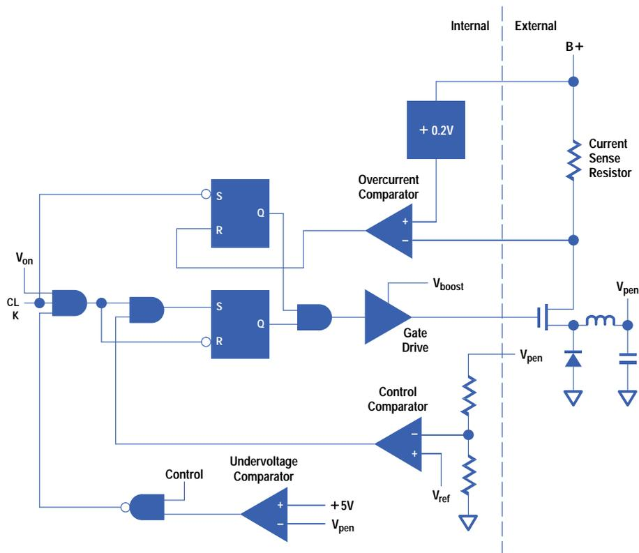
**Fig. 3.** Block diagram of the dc-to-dc converter.
