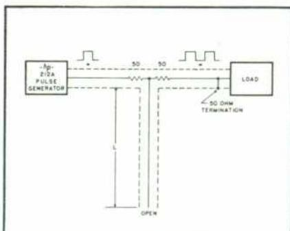
Figure 5. Circuit For Generating Double Pulses.
