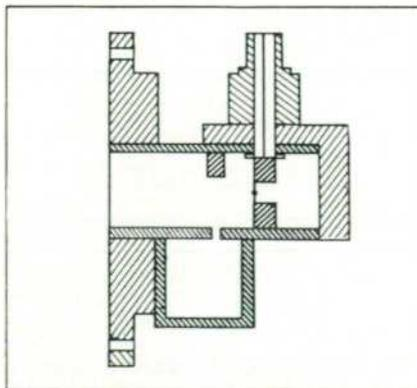
Fig. 3. Simplified cross-sectional drawing of Model 487A waveguide mount.
