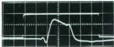
Oscilloscope showing simplicity of scope presentation obtainable when Delay Generator and Pulse Duration Unit are used to establish a visual go-no-go gage for rapid tests on delay devices. Illustration shows a delay line whose delay is within tolerance as marked by rectangular pulse. Sweep time is 1  $\mu\text{sec}/\text{cm}$  but delay preceding sweep start can be any amount up to 10,000  $\mu\text{secs}$ .
