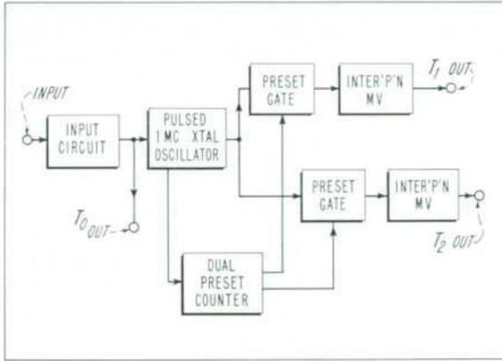
Fig. 3. Basic circuit arrangement of Digital Delay Generator.
