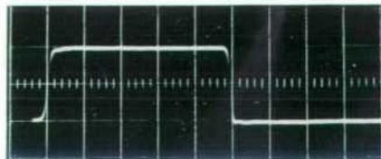
Fig. 8. Oscilloscope showing typical quality of pulses from 90-ohm output of 219C Pulse Duration unit (0.1  $\mu\text{sec}/\text{cm}$  sweep). Pulse is available at either polarity and of duration  $T_0$  to  $T_1$  or  $T_1$  to  $T_2$ .
