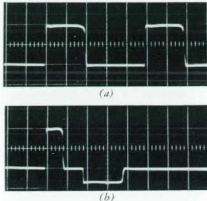
Fig. 7. (a) Oscilloscope showing typical quality of output pulses from Model 219B Dual Pulse Unit (1  $\mu\text{sec}/\text{cm}$  sweep). Pulses can each be obtained from separate outputs or from common output as shown. Polarity, width, amplitude and spacing of pulses from 219B output unit are individually adjustable as indicated by (b).
