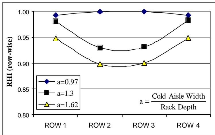
Figure 8: Variation of row-wise RI with cold aisle geometry parameter "a"
