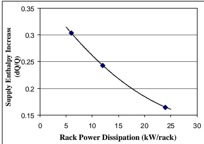
**Figure 13:** Supply Air Enthalpy Increase vs. Data Center Power Dissipation
