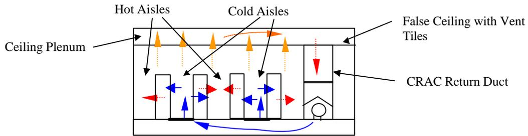
**Figure 2.** Typical Under Floor Air Cooling Data Center Configuration with Ceiling Return
