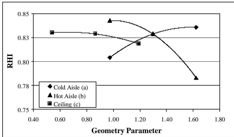
**Figure 11:** Variation of RHI with Geometry Parameters for Ceiling Return
