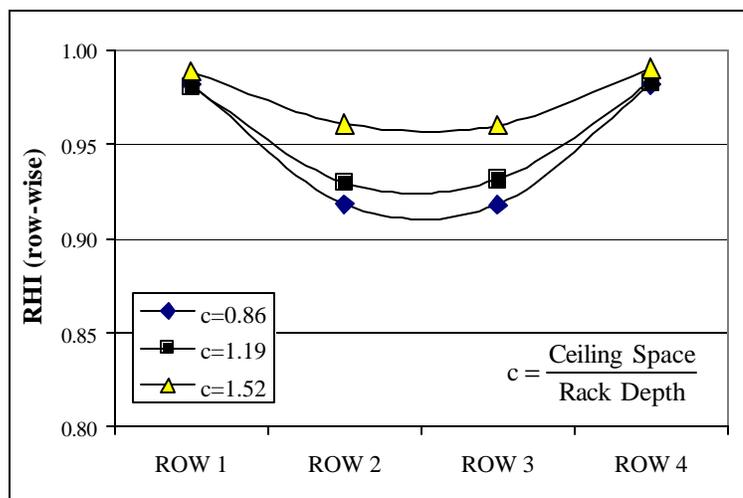
Figure 9: Variation of row-wise RI with ceiling space geometry parameter "c"
