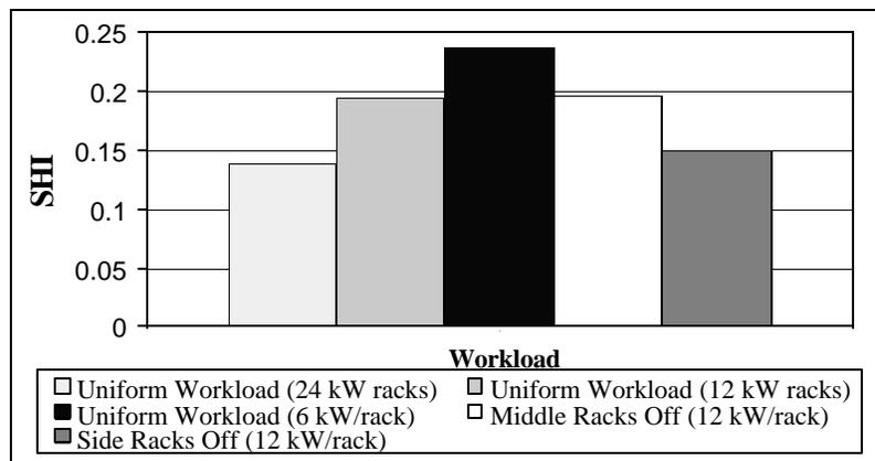
**Figure 12:** Variation of SHI with Data Center Equipment Workload
