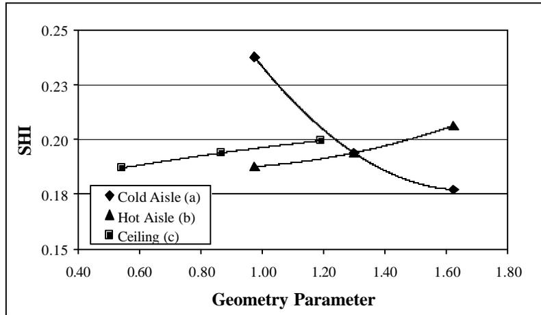
**Figure 10:** Variation of SHI with Geometry Parameters for Ceiling Return
