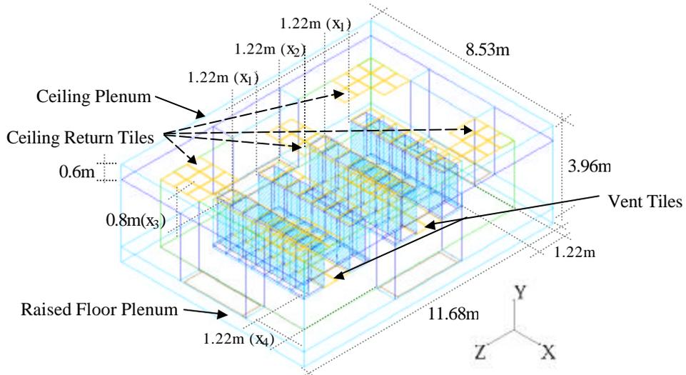
**Figure 4:** Base Case layout for ceiling return infrastructure
