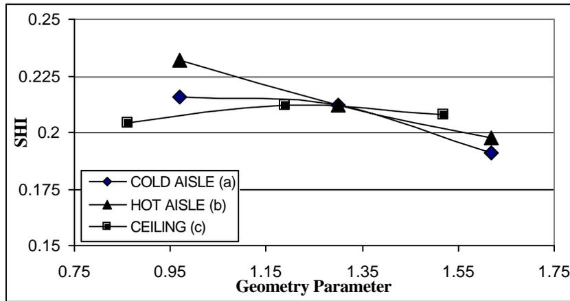
**Figure 6:** Variation of SHI with Geometry Parameters for Room Return
