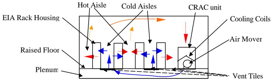
**Figure 1.** Typical Under Floor Air Cooling Data Center Configuration with Room Return
