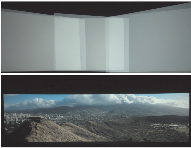
Fig. 10. The proposed paradigm automatically corrects the inherent geometry, color, luminance, and black offset variations among six projectors in a three-wide, two-deep hybrid configuration (top) to create a seamless and high quality result on a 16' wide screen (bottom).
