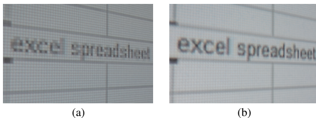
Fig. 9. Experimental results with four superimposed projectors: (a) single aliased subframe (contrast enhanced for visibility) versus (b) super-resolved output. Note the resolution enhancement as well as brightness gain of the superimposed result.
