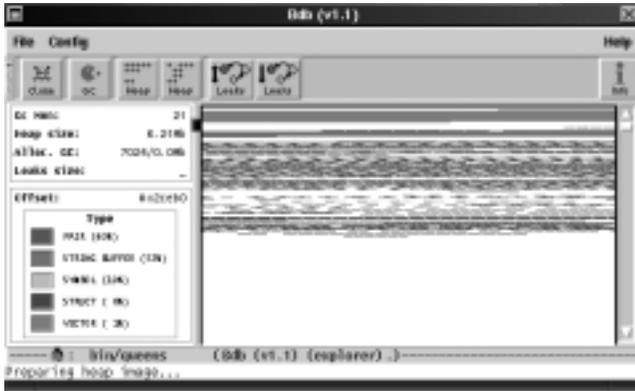
Figure 6: An heap view according to object types
