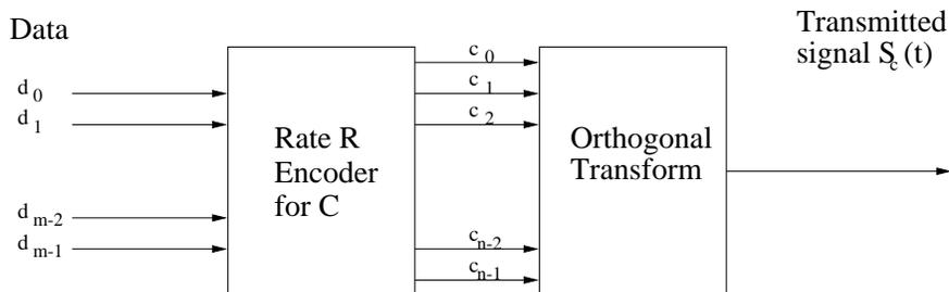
**Fig. 4.** Model for communication by orthogonal transforms with coding. Here  $R$  denotes the rate of the code  $C$  and  $m = Rn$  is the number of data bits input to the encoder
