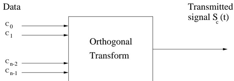
Fig. 1. Model for communication by orthogonal transforms
