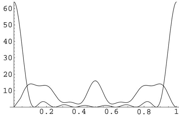
**Fig. 2.** (Envelope) powers of OFDM signals for  $c = 00000000$  and  $c = 00011101$ , with  $t$  normalised to  $[0, 1]$  by taking  $\Delta f = 1$
