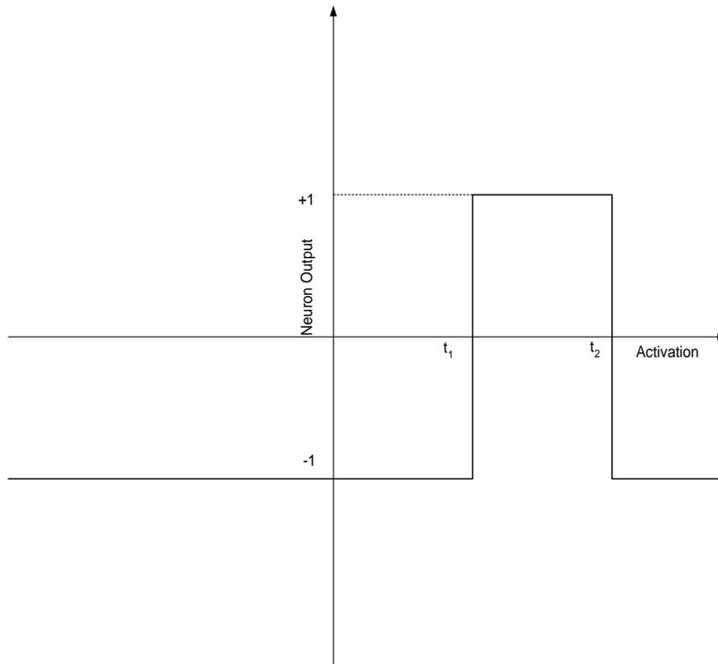
Figure 1: The transfer function for the bithreshold neuron model. This type of characteristic can be obtained by tying the outputs of two open-collector amplifiers, one of which compares the input with  $t_1$  and the other with  $t_2$ .
