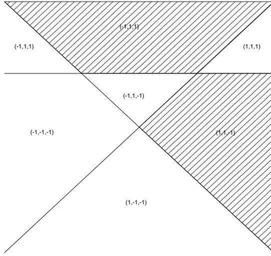
Figure 2: Example of a decision region in 2-dimensional input space implementable by a 2-layer network with 3 first layer neurons and a bithreshold neuron output (without further addition of first layer neurons to the existing network) that is not implementable by a 2-layer perceptron with 3 first layer neurons with threshold output. The vertices of the 3-cube that correspond to the basic convex polytopes are also indicated in the figure.
