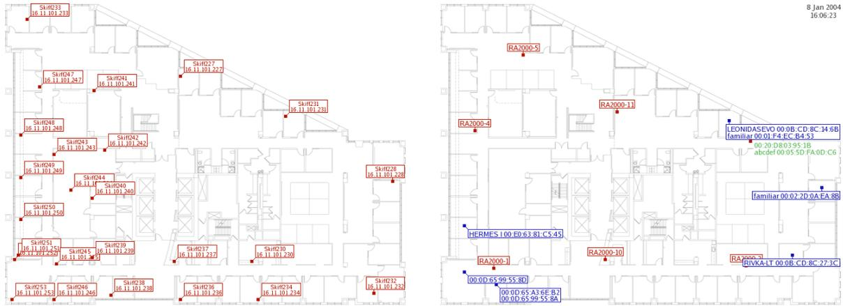
Figure 4: Scanner locations (left), and snapshot of live targets being tracked (right). The 8 blue boxed targets have been located to a single room; the 2 targets in green have approximate locations. The 7 red “RA2000-#” targets are access points. Another 43 targets (not shown) have been identified as being outside of this building.
