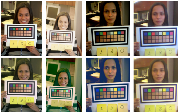
Fig. 2. Images before (top row) and after (bottom row) color correction, for all four cameras. Left to right: HP850, Nikon D1, iPAQ, web-cam. Transforms based on skin patches only.
