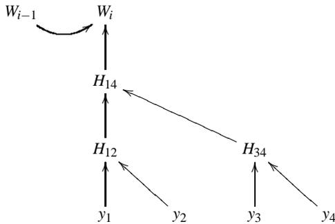
Figure 1. Hash-Linking using a Merkle hash tree
