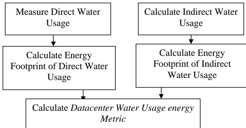
**Figure 8: Flowchart for calculation of data center water usage energy metric.**
