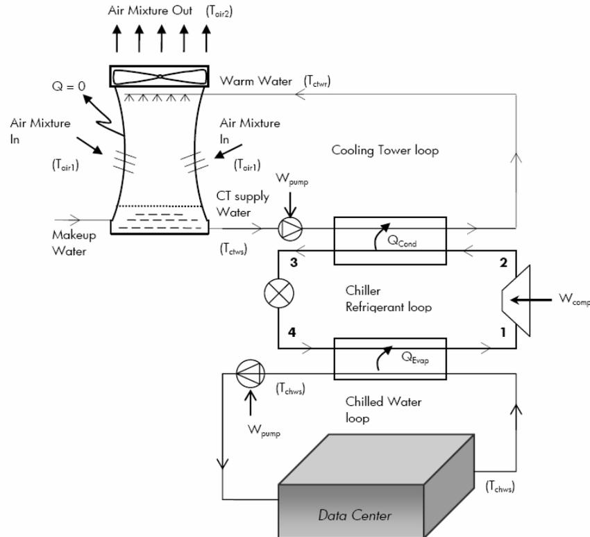
**Figure 3: Data Center Facility Cooling infrastructure**
