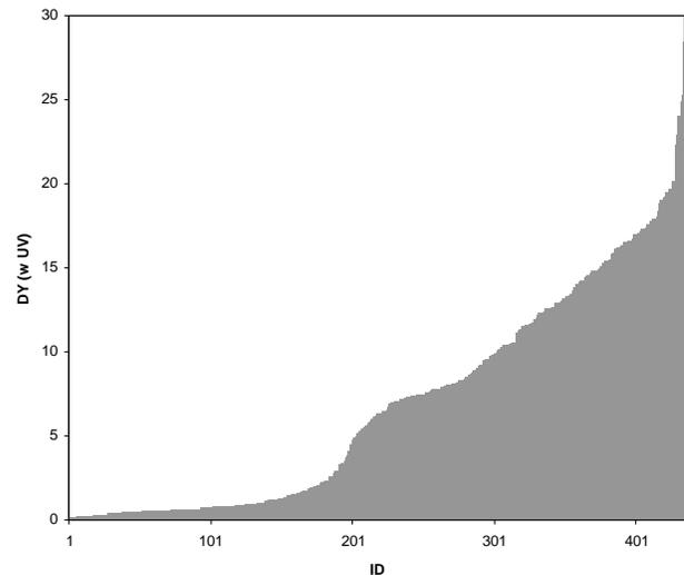
Figure 8. Sorted fluorescence measurements for the print substrate database.
