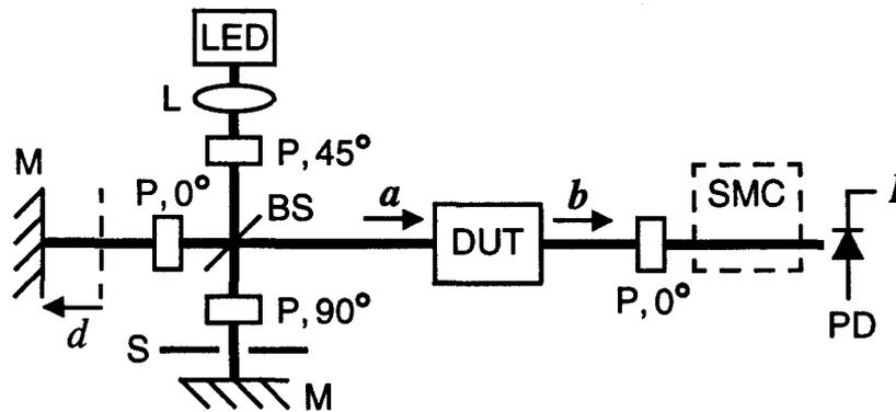
**Figure 1.** Apparatus used for measurement of polarization mode dispersion using frequency scanning and interferometry. LED: light emitting diode; L: lens; P: linear polarizer; BS: beamsplitter; M: mirror; DUT: device under test; SMC: scanning monochromator; PD: photodiode.
