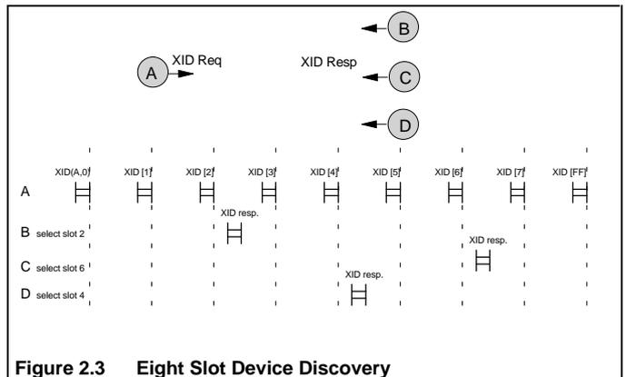
Figure 2.3 Eight Slot Device Discovery
