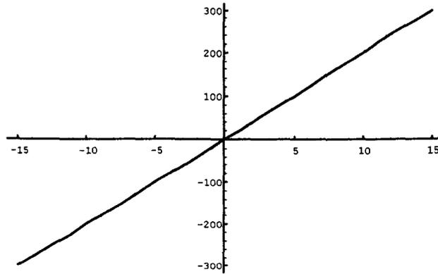
Figure 7: Simulated output of dual stripe magnetoresistive head. Function plotted is  $V=[-(x-x_0)^2]-[-(x+x_0)^2]$ : abscissa represents the applied field; the ordinate, the voltage response (arbitrary units). Note the linearity of the response.
