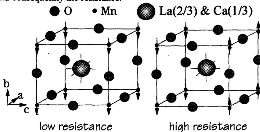
Figure 15: Crystal structure of  $\text{La}_{0.67}\text{Ca}_{0.33}\text{MnO}_{3+\delta}$ . Center of unit cell: La and Ca ions; corners: Mn ions; edge center: oxygen ions. Magnetization of the Mn ions (for 0% Ca) is indicated in the high resistance state diagram. Canting of the spins, ferromagnetism and conductivity are induced by doping with  $\text{Ca}^{2+}$ . See text for clarification.
