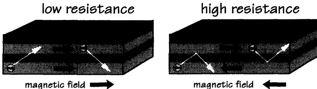
Figure 10: Schematic of the principle of operation of a spin valve system. Two magnetic layers (gray) are separated by a non-magnetic spacer (black). The magnetization of the top layer is pinned by exchange coupling to an antiferromagnet layer (pattern), while the magnetization of the bottom magnetic layer (sense layer) is free to rotate in response to a magnetic field.
