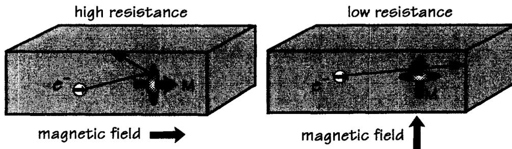
Figure 3: Schematic demonstrating the physical origins AMR. Shaded ovals represent the scattering cross-sections of the bound electronic orbits. When the orbits (and applied field) are transverse to the current direction, the electron scattering cross-section is reduced, giving a low resistance state.
