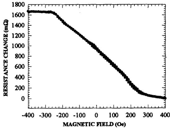
Figure 12: Output of HP spin valve head. Note linearity of signal, lack of hysteresis and lack of noise in the operating region.
