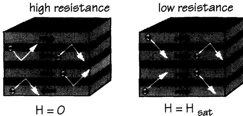
Figure 9: Schematic of the high and low resistance states of the GMR multilayer systems.
