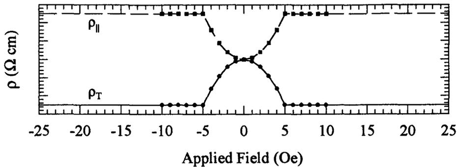
Figure 2: Schematic representation of anisotropic magnetoresistance in permalloy for field applied parallel ( $\rho_{\parallel}$ ) and transverse ( $\rho_{\perp}$ ) to the current direction.
