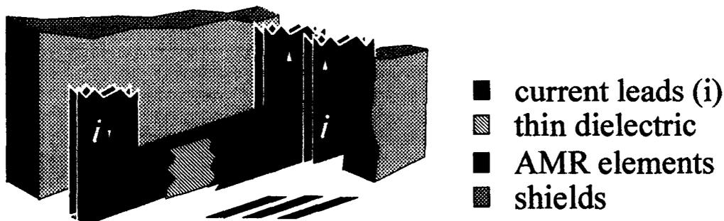
Figure 6: Schematic of Dual Stripe MagnetoResistance head. The magnetic fields generated by the current in each stripe bias the other stripe.
