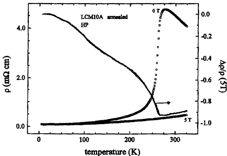
Figure 16: Resistivity at  $H = 0$  and 5 Tesla (squares), and magnetoresistance effects of CMR samples grown at HP Labs. Note a decrease in resistance of over 90% at room temperature. Also, the magnetoresistance effect is relatively constant over a temperature range of  $\sim 50$  degrees.
