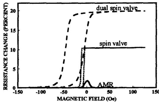
Figure 13: Comparison of the percentage of resistance change for an AMR, spin valve and dual spin valve heads.
