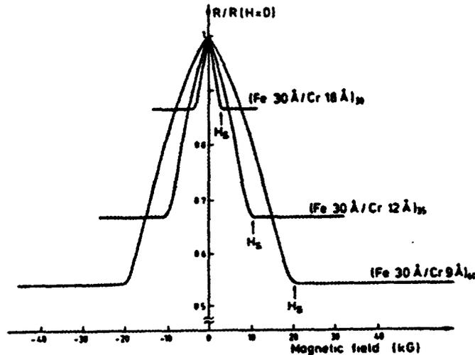
Figure 8: Giant Magnetoresistance effect as reported by Baibich *et al.*
