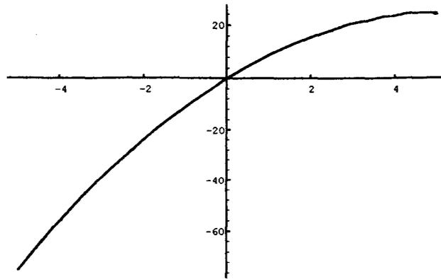
Figure 5: Simulated output of a SAL biased AMR recording head. Function plotted is  $V = -[(x-x_0)^2 + y_0]$ ; the abscissa represents the applied field; the ordinate, the voltage response (arbitrary units). Note the non-linearity of the response - the magnitude is less for positive applied fields than for equally large negative applied fields - giving asymmetric peak heights in the read back signal.
