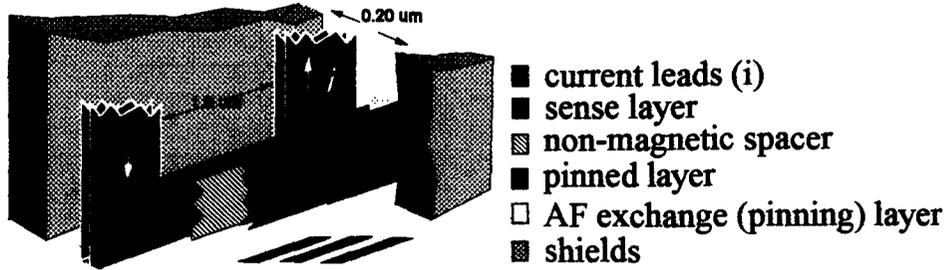
Figure 11: Schematic of a spin valve read head. The magnetization of the pinned layer (pointing up) is set 90 degrees to the zero field state of the sense layer (aligned along the track width). Positive fields decrease the angle between the two magnetizations, decreasing the resistance; whereas, negative fields increase the angle and the resistance.
