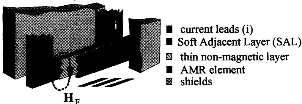
Figure 4: Schematic of recording head utilizing the SAL biasing technique. The fringing field from the SAL layer rotates the magnetization of the AMR element, effectively biasing the head.
