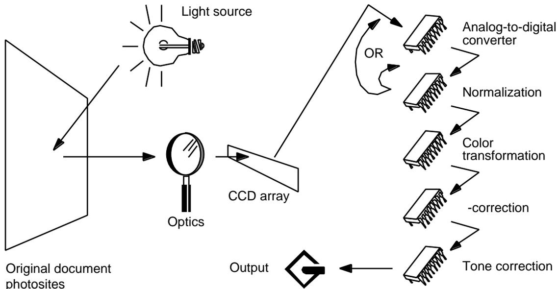
**Figure 1. Conceptual pixel flow in a typical scanner. The order of the processing blocks on the right can be different.**
