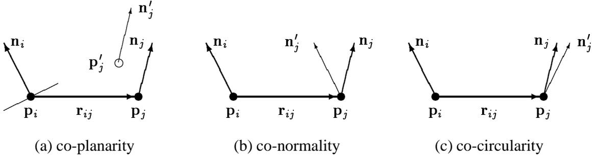
Figure 3: The three oriented particle interaction potentials. The open circles and thin arrows indicate a possible new position or orientation for the second particle which would lead to a null potential.
