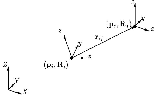
Figure 2: Global and local coordinate frames. The global interparticle distance  $\mathbf{r}_{ij}$  is computed from the global coordinates  $\mathbf{p}_i$  and  $\mathbf{p}_j$  of particles  $i$  and  $j$ . The local distance  $\mathbf{d}_{ij}$  is computed from  $\mathbf{r}_{ij}$  and the rotation matrix  $\mathbf{R}_i$ .
